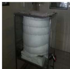
Figure 2: Insulation of Ceramic Fibre Blanket
