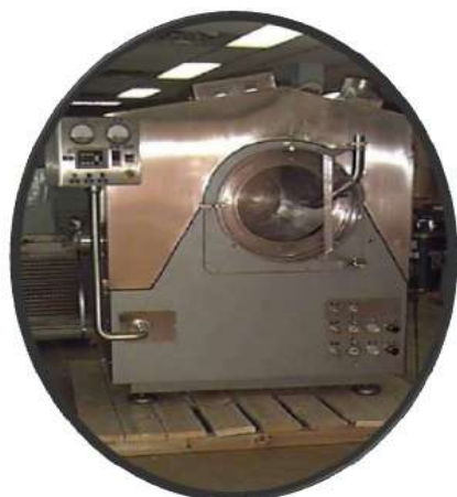
Figure 1. Side vented tablet coating pans
