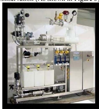
Figure 3. Advanced automatic Coating in Place (CIP) and Washing in Place (WIP) systems
