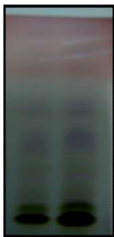
Fig-9: TLC plate of ethanolic extract in duplicate and Scanned after spraying with anisaldehyde reagent
