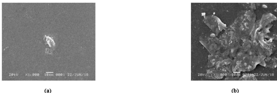
Figure 2: Scanning electron microscopy image of polystyrene plastic film surface, (a) before biodegradation test, (b) after biodegradation test using bacterial isolates obtained from the soil of Jayawijaya Mountains, Papua in Agar Nutrient medium
