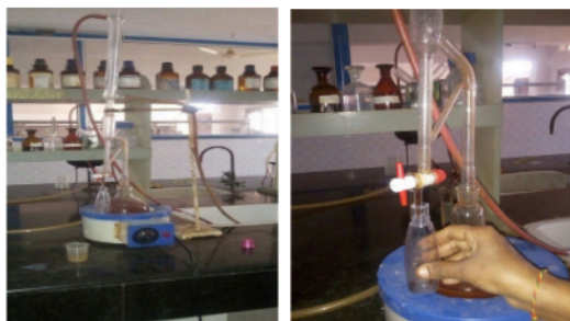
Figure 1: Extraction of cinnamon oil by steam distillation
