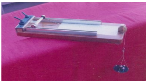
Figure 2: Tensile strength measuring apparatus
